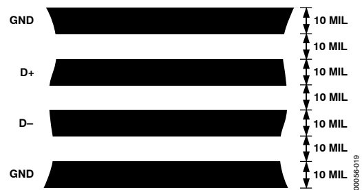
Figure 19. Arrangement of Signal Tracks
